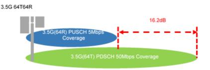
Figure 9: Uplink Coverage difference between C-Band and LTE 1800
