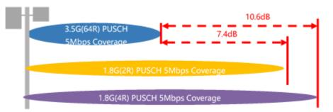
Figure 10/11: Combining DL on C-band with UL on sub-3 GHz band, Field Test Result
