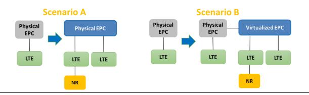
Scenario A is the easiest way, but it has also brought a big drawback. When evolving to 5G SA, this physical EPC based on dedicated hardware cannot be used in a virtualized environment. This scenario depends on the capabilities of the existing network equipment vendors. Compared to scenario A, scenario B can be smoothly evolved to the target network through the expansion of virtualized EPC.
