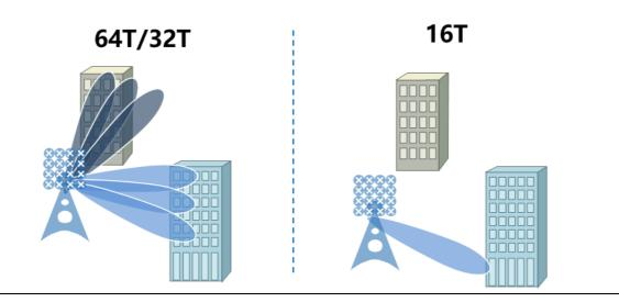
5G network deployment needs to fully consider performance, cost, space and weight limitation, etc. The most cost effective configuration, 64T, 32T or 16T may be different for different deployment scenarios due to the different performance benefits in the scenarios, respectively. 64T/32T tends to perform better in dense-urban high-rise scenarios and hence may be more cost efficient, whereas 32T or 16T tend to be more cost efficient in urban and suburban scenarios.
